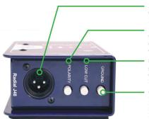
XLR OUT balanced, mic-level output used to feed a mixer or a mic preamp.
