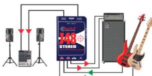
**J48 Stereo with two different instruments**
