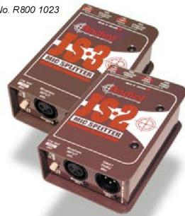
The Radial JS•2 and JS•3 are Jensen transformer-equipped mic splitters that allow a balanced source to drive multiple destinations via standard XLR connectors. These passive devices feature a premium nickel laminated core transformer for exceptionally low harmonic distortion without the usual phase shift caused by lesser steel core transformers.
