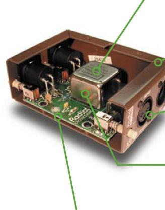
**JENSEN** audio transformers provide 100% isolation to eliminate noise caused by ground loops, and they sound great!
