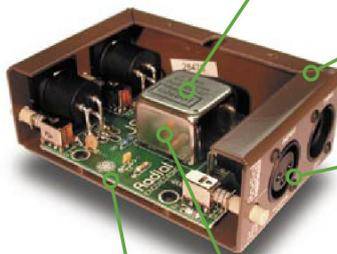
**JENSEN** audio transformers provide 100% isolation to eliminate noise caused by ground loops, and they sound great!
