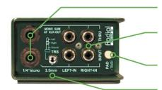
1/4" INPUT and THRU-PUT standard connection for bass, guitar and keyboard.
