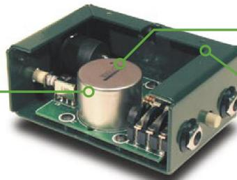
**MU-METAL SHIELD** for protection against radio frequency and electromagnetic interference.
