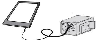
For stereo operation, connect the left and right 1/4" TRS balanced outputs from the SB-5 to two mic inputs on the PA system. In most cases you will find that using a pair of 1/4" TRS to XLR-M adaptor cables to be the best choice. The SB-5's output is mic level and therefore should be connected to a microphone input. Set the two PAN controls on the mixer hard left and hard right for full stereo performance. Adjust the level to suit.
